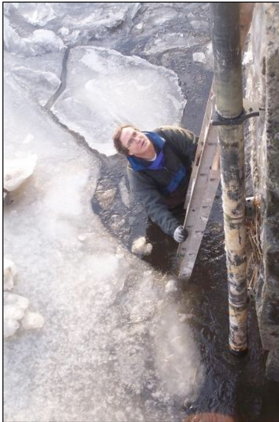
Hap Garritt removing an oxygen logger from Middle Road Bridge in winter.
